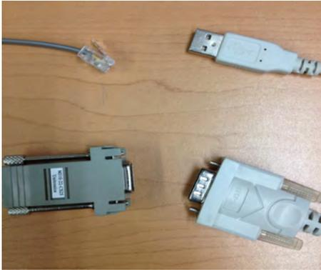
Figura 4.10: RJ-11-Serial\Serial-USB.
