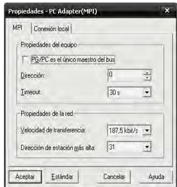
Figura 3.10: PG/PC Interface SetUp.
