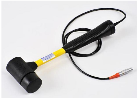
Figura 1.2. Martillo instrumentado ( www.testconsult.co.uk )
