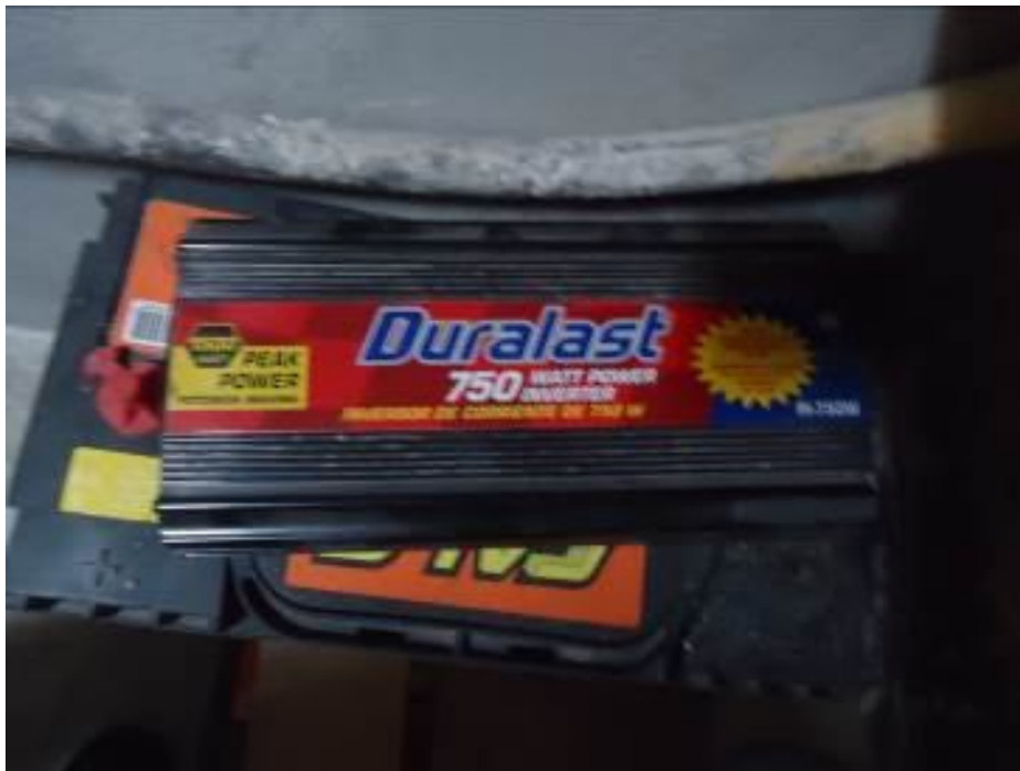
Figura 3.19 Inversor C.D a C.A.
