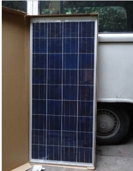
Figura 3.16 Modulo solar de 130 watts.
