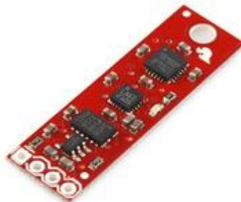
Figura 5.13 IMU Sensor Stick.
