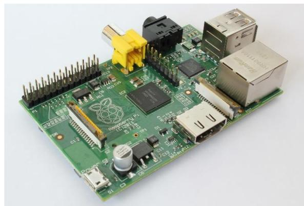
Figura 2.3 Tarjeta Raspberry Pi Mod B.
