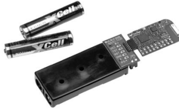
Figura 4.20 Transceiver Texas ez430-RF500 [47]
