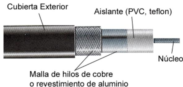
*Figura 1.8. Cable coaxial*
