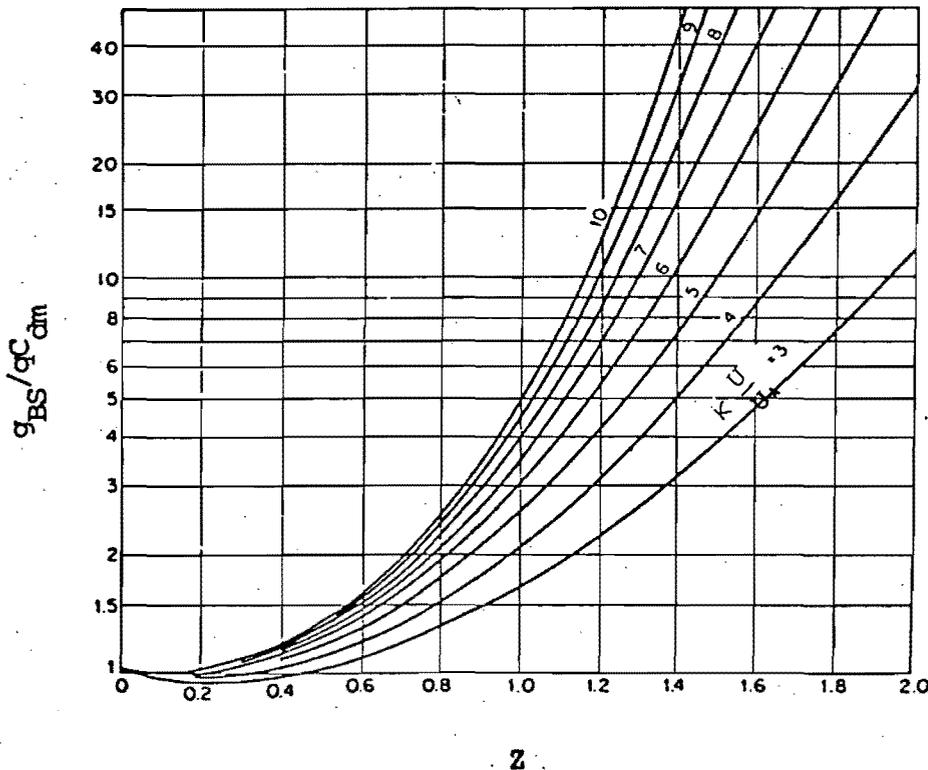
Fig. 4.4.1 FUNCION  $g_{BS}/q C_{dm}$  EN TERMINOS DE  $\kappa \frac{U}{U_*}$  Y  $z$  (SEGUN BROOKS 1963)
