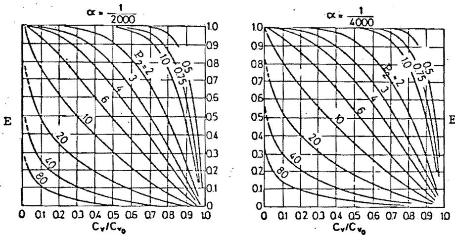
Fig. 2.3.3 VARIACION DE LA CONCENTRACION VOLUMETRICA RELATIVA ( $C_v/C_{v0}$ ), PARA DISTINTOS VALORES DE E Y  $P_2$ , Y PARA RUGOSIDADES RELATIVAS  $\alpha = 1/2000$  Y  $\alpha = 1/4000$
