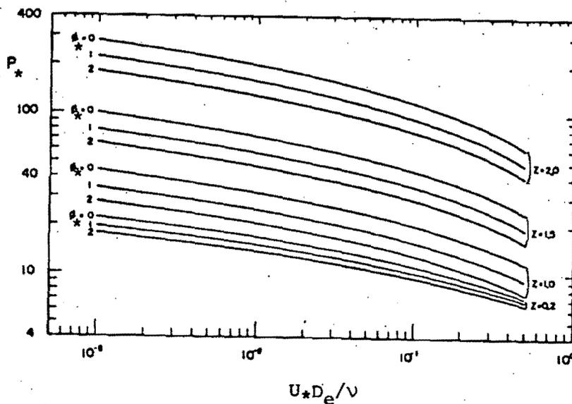
Fig. 4.9.1. FUNCION  $P_*$  EN TERMINOS DE  $K_S/d$  Y  $Z$ , PARA  $a/d = 0.05$  Y  $B' (U_* K_S / \bar{v}) = 8.5$
