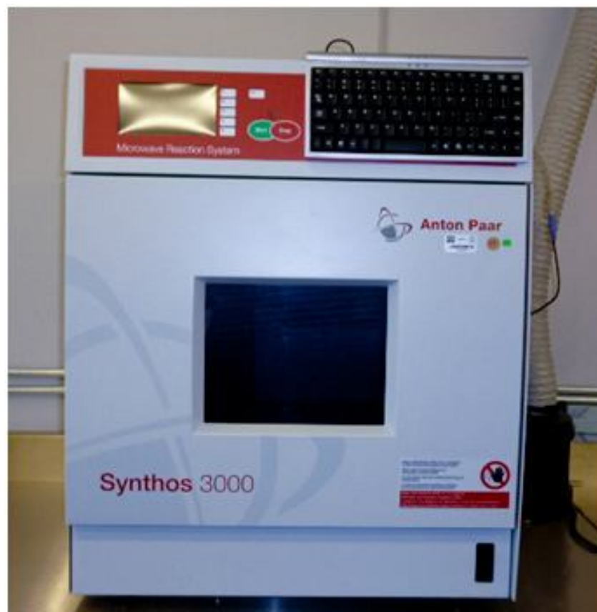
Figura 5. Horno reactor de microondas Anton Paar Synthos 3000.
