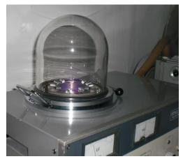
Figura 41. Ion-sputter JEOL modelo JFC-1100E.
