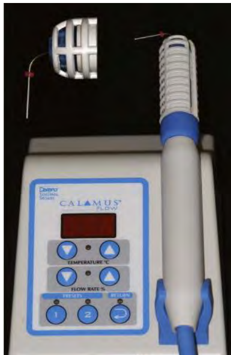
Fig.24: Unidad termoplástica Calamus (DENTSPLY Tulsa Dental Specialities, Tulsa, OK) para calentar e inyectar gutapercha. (Tomado de Hargreaves Cohen's Pathways of the Pulp, 10th Edition)
