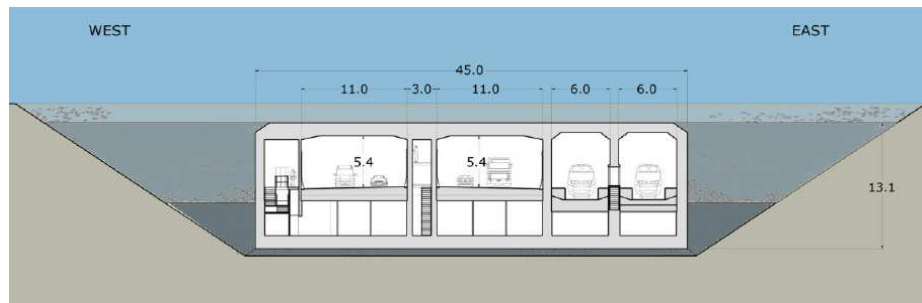
Figure 2.23(b) Special Cross section of the Fehmarn Belt IMT (De Wit et al., 2012)
