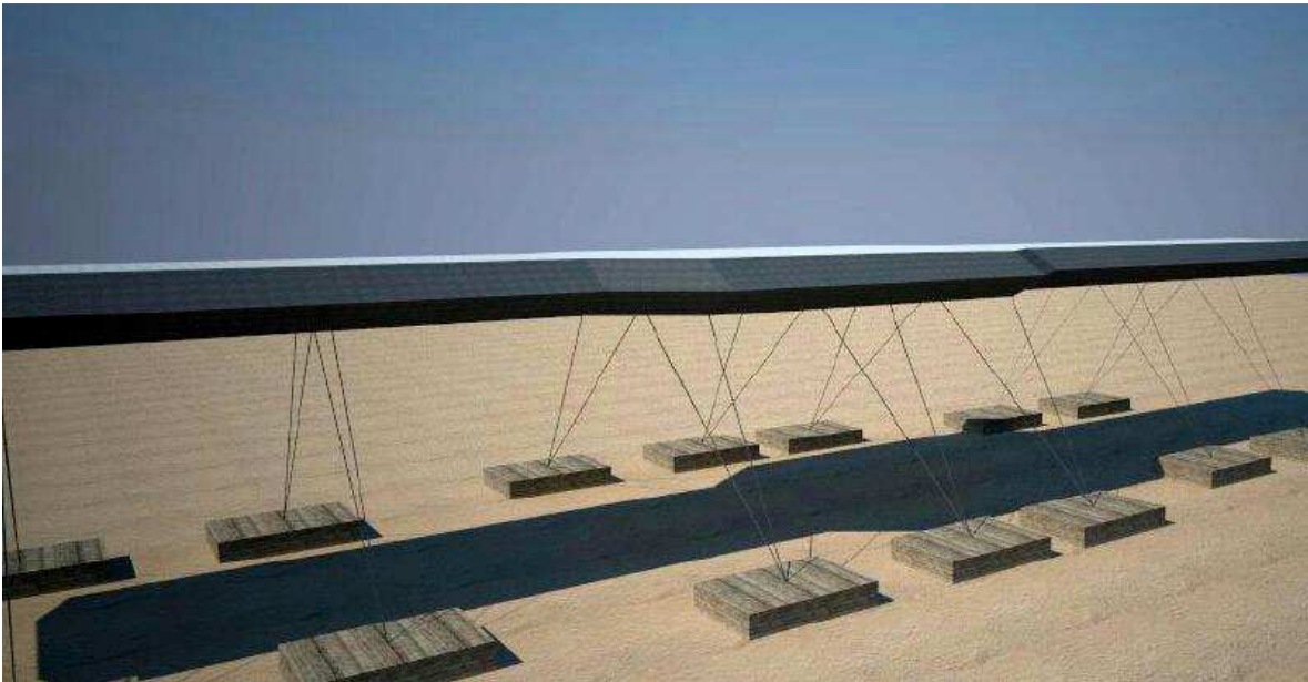
Figure 4.54 3D rendering of the longitudinal alignment of the SFT of the Gulf of California
