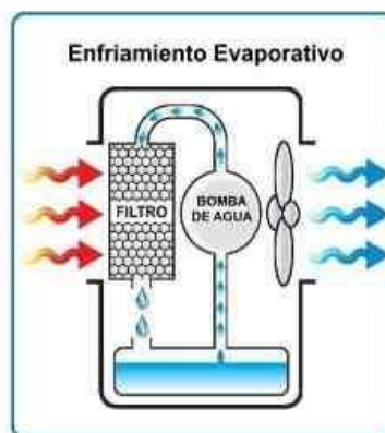
FIGURA 3.1 ESQUEMA DE FUNCIONAMIENTO ( http://voices.yahoo.com/how-clean-mold-mildew-out-window-air-conditioner-5822060.html ).
