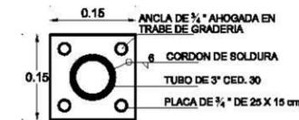
**D-2 DETALLE DE PLACA DE ANCLAJE**
