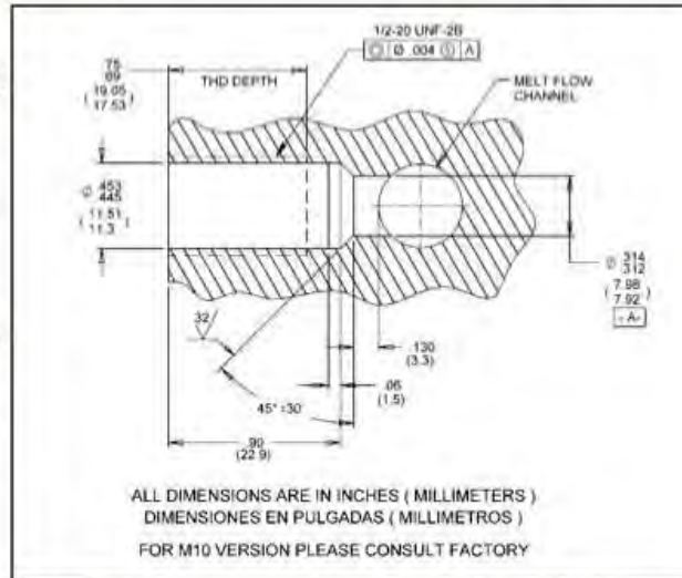
FIGURE 1 - Recommended Mounting Well (1/2-20 UNF) FIGURA 1 - Agujero de Montaje Recomendado (1/2-20 UNF)
