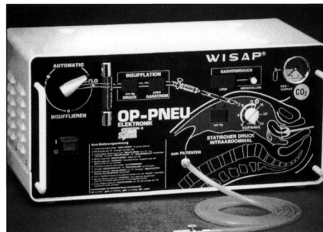
Figure 2. Semm's electronic insufflator. (Figure C-4 in Highlights in the History of Laparoscopy .)
