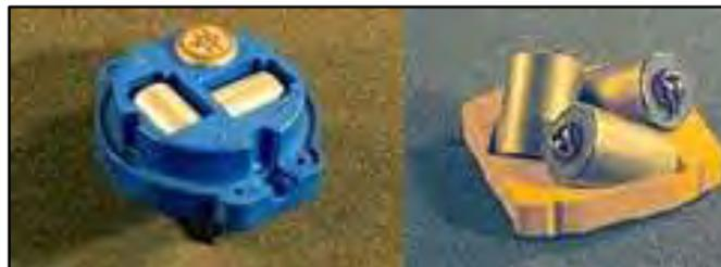
Figura 4.17\_Sensor digital 3C (Tomado de CREWES, 1998; ION GX Technology, 2009).
