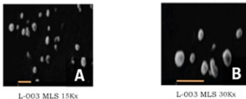
Figura 6: Micrografías de MLS Lote 003, 10% Compritol® 888. Aumento: (a) 15,000x; (b) 30,000x. Barra=10 µm.
