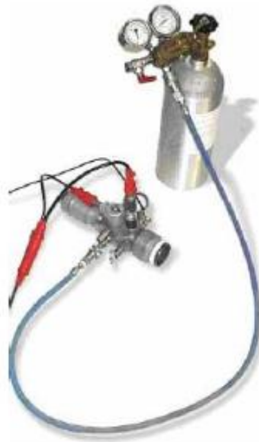
Figura3-5. Pistola remota conectada al well analyzer. Fuente: Echometer company.
