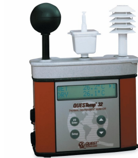
(b) 3M QUESTemp Heat Stress Monitor with black globe thermometer that reads radiant temperature.
