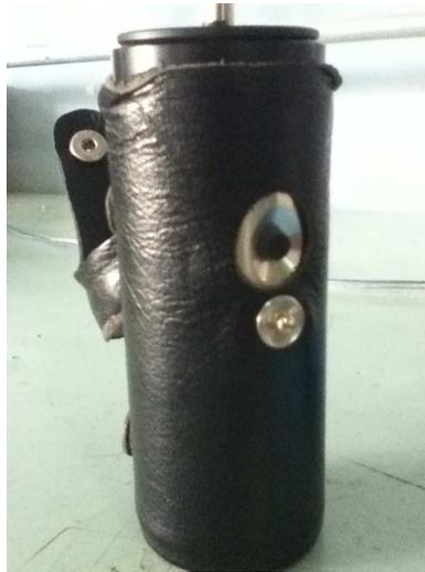
Figura 4.5: Calibrador *Sound Level Calibrator Type 4230*.
