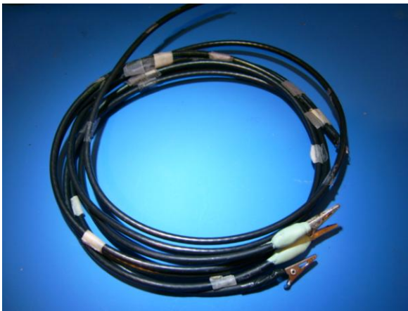
Figura 5.1 Cable coaxial RG59
