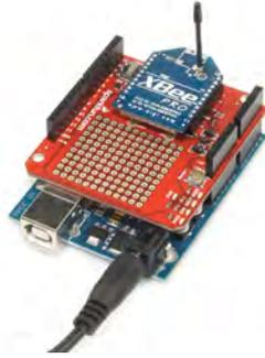
Figura 5.11: Xbee shield
