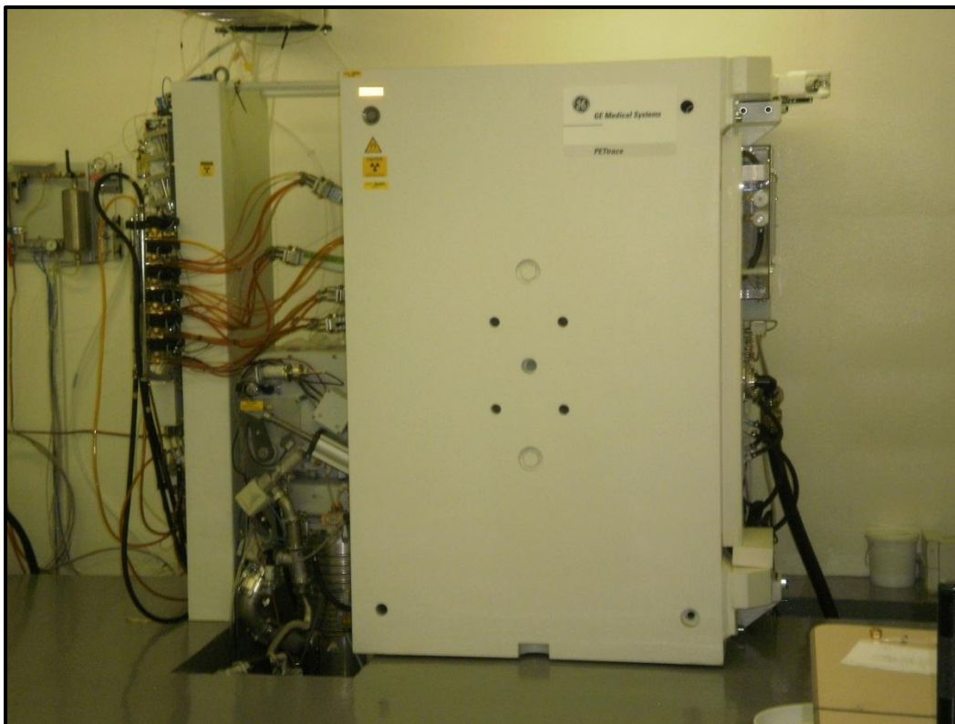
Fig. 3.2 Ciclotrón General Electric Medical Systems PET trace 6, 17 MeV protones/8 MeV deuterones.
