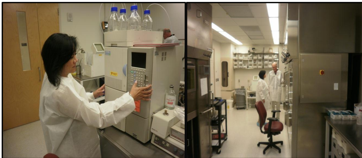
Fig. 3.7 Sistema HPLC Nucleosil 120-7 C18 (250 mm X 4.6 mm).
