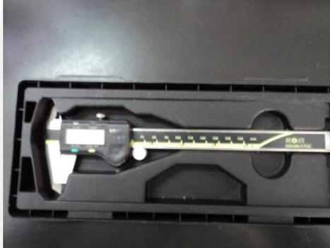
**Fig.22**Vernier digital Mitutoyo.
