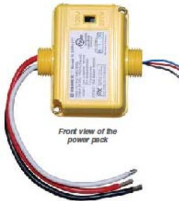
The Square D® Power Pack supplies low voltage power to Square D ceiling and wall mounted occupancy sensors, and employs a heavy duty 20A relay to switch lighting and HVAC loads based on a control signal received from the occupancy sensor. The power pack accepts both 120V and 277V input and supplies up to 100mA at 24VDC.
