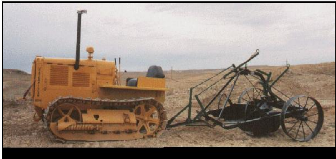
1934 Cat 22 pulling a Miskin Model D Scraper
