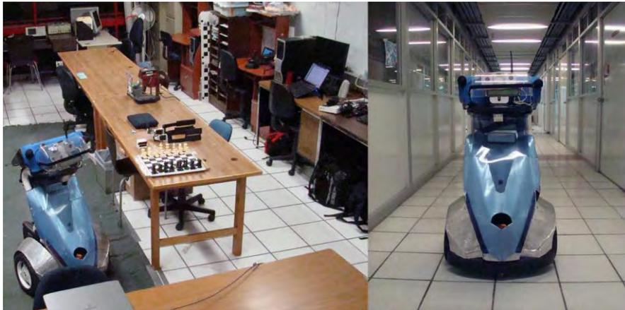
In order to minimize the initial pose error when building the map, the floor tiling (at every 30 cm) was used to set the robot at every 2.10 meters  $\pm$  3 centimeters, performing four scans at the absolute headings of zero, 90, 180 and 270 degrees at every robot stop (Fig. 24, left). This process took about 2 hours for scanning the 50 meters long corridor and the 5  $\times$  7 m Biorobotics Laboratory.
