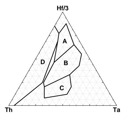
Figure 7. The Th-Ta-Hf/3 ternary diagram (Wood 1980) for island arc basalt (IAB; field D), within-plate basalt (WPB; field C), normal type mid-ocean ridge basalt (N-MORB; field A), and enriched type mid-ocean ridge basalt (E-MORB; filed B).
