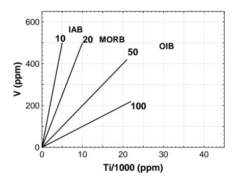
Figure 3. The Ti/1000-V bivariate diagram (Shervais 1982) for island arc basalt (IAB; Ti/1000-V equi value of 10-20), ocean-island basalt (OIB; Ti/1000-V equi value of 50-100), and mid-cean ridge basalt (MORB; equi value of 20-50).
