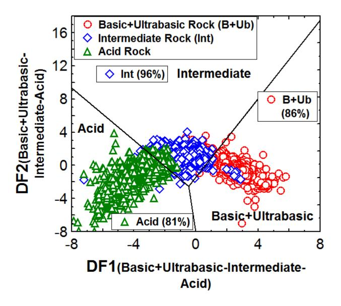
Figure 1 New discriminant-function based multi-dimensional diagrams for the classification of igneous rocks from basic+ultrabasic (B+Ub), intermediate (Int), and acid rocks, showing samples from the data set.
