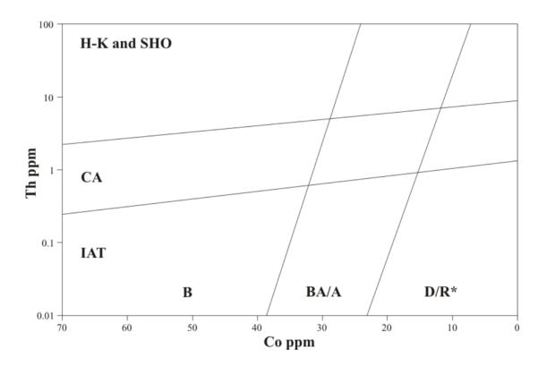
Figure 15. Co-Th, (Hastie *et al.* 2007) classification diagram for altered igneous rocks. The rock type abbreviations in Co-Th diagram are: B-basalt; BA/A-basaltic andesite/andesite; D/R\*-dacite/rhyolite/latite/trachyte; IA-T-island arc tholeiite; CA-calc-alkaline; and H-K and SHO-high-K and shoshonite.
