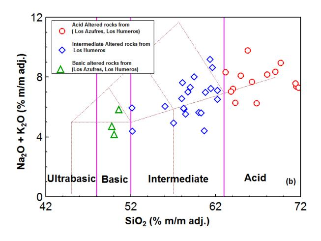
Figure 2b. Total Alkali versus Silica (TAS) classification diagram for altered rocks, showing samples from the five case studies. The solid pink lines represent field boundaries for ULTRABASIC–BASIC–INTERMEDIATE–ACID (1+2-3-4) fields.
