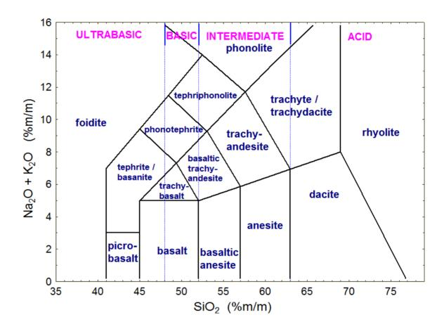
Figure 14. The chemical classification and nomenclature of volcanic rocks using the total alkali versus silica diagrams of Le Bas *et al.* (1986).
