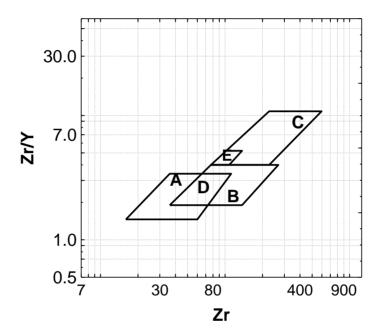
Figure 2. The Zr-Zr/Y bivariate diagram (base 10 log-log scales; Pearce and Norry 1979) for island arc basalt (IAB; field A), within-plate basalt (WPB; field C), mid-ocean ridge basalt (MORB; field B), overlape region of IAB and MORB (IAB+MORB; field D), and WPB and MORB (WPB+MORB; field E).
