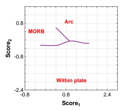
Figure 11. The Score<sub>1</sub>-Score<sub>2</sub> diagram (Butler and Woronow 1986) for arc (IAB), within-plate (WPB), and mid-ocean ridge (MORB).
