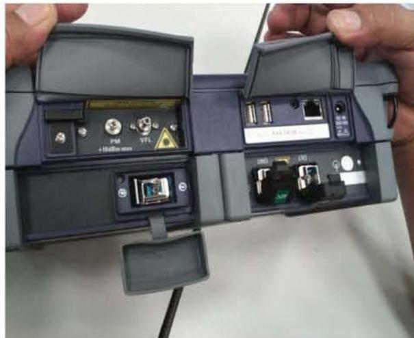
FIGURA 3.24 OTDR-JDSU c) Módulos
