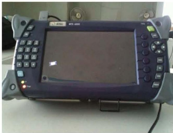
FIGURA 3.24 OTDR-JDSU a) Parte Frontal.
