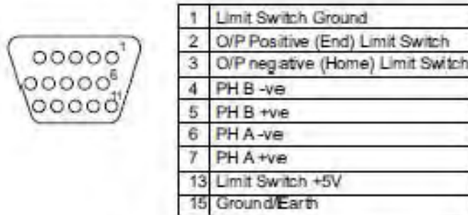
Fig. 4.8 Motor pin out details
