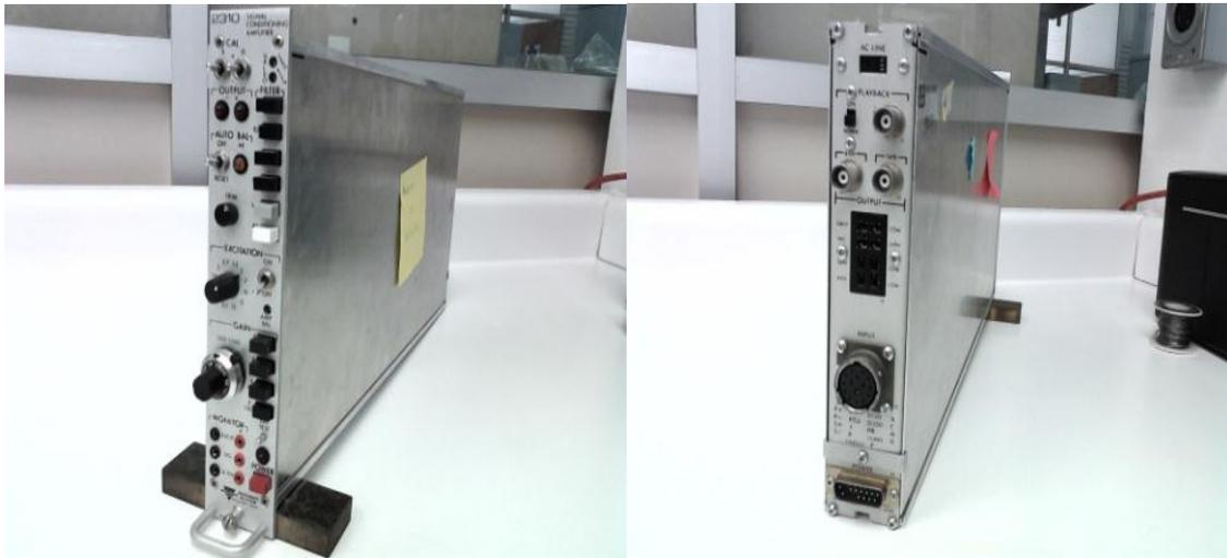
Figura 3.33 Signal Conditioning Amplifier System 2310.
