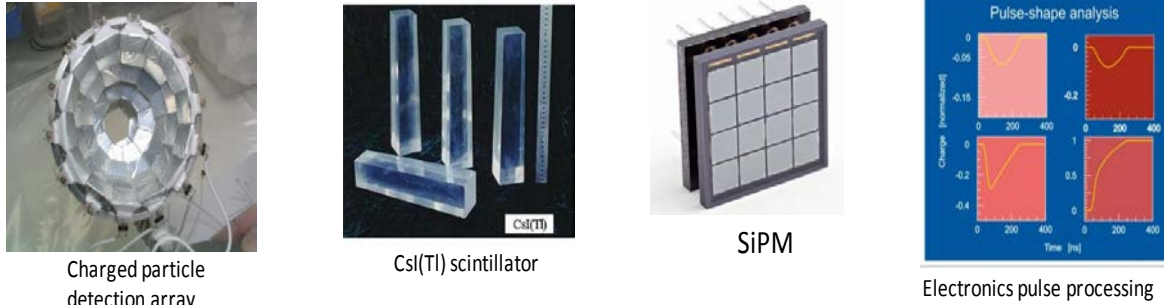
Figure 3.4: Prototype for charged particle detection consisting of a CsI(Tl) scintillator optically coupled to a SiPM for the electronics read out.
