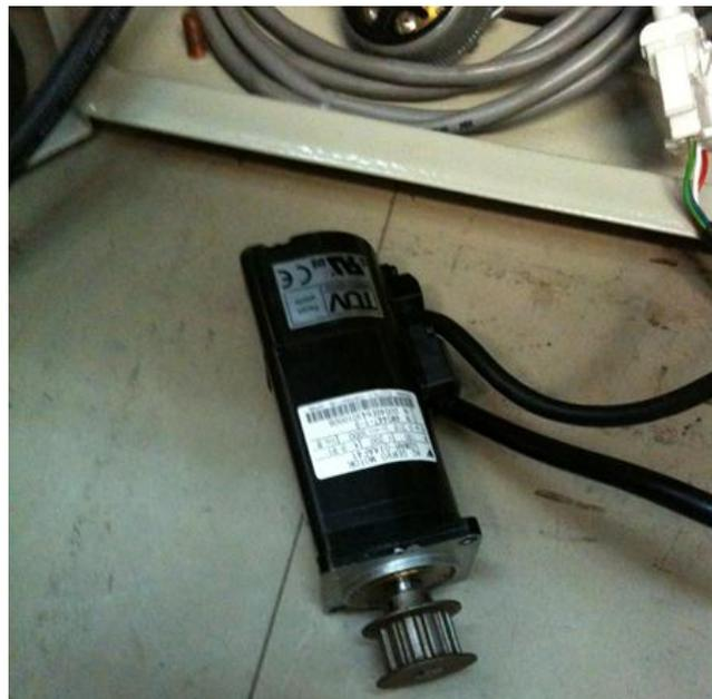
**Figura 2.16. Servomotor SGMAH 01AAF.**
