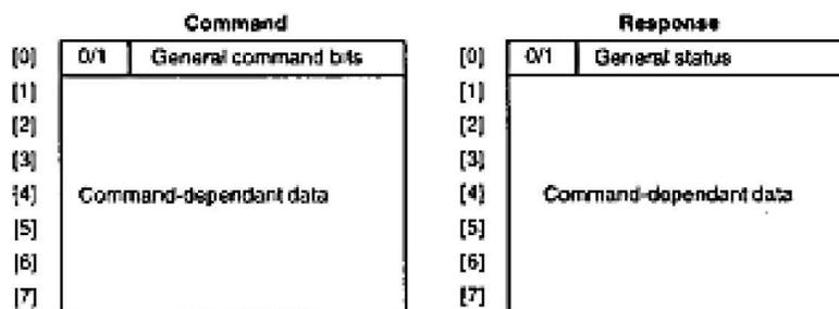
Both the command and response data are separated into two sections. Byte 0 is a general area and bytes 1 to 7 make up the command-dependant data area. The command-dependant data area depends on the two types of commands, move commands and set/read commands. The type of command is defined by the most-significant bit of byte 0.
