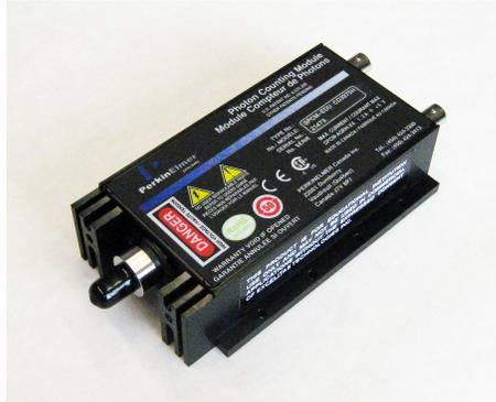
Figura A.3: Perkin Elmer Photon Counting Module SPCM-EDU.
