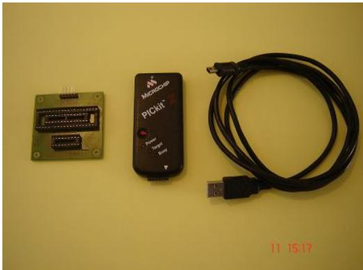
Figura 6.17 Programador de PIC's **PICKit 2 v2.61**
