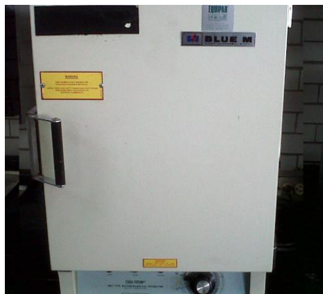
Figura 14. Incubadora (Dry Type Bacteriological Incubator).
