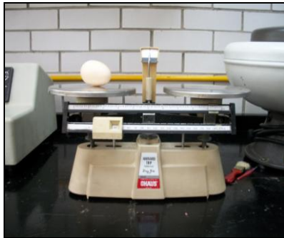
Figura 8. Balanza Granataria Harvard Trip Balance 2 kg-5lb.
