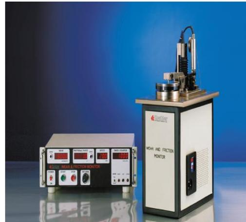
**Figura 76.** Vista Frontal probador Pin- on- disc, [46].
