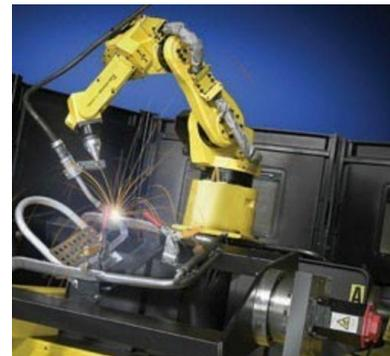
Figura 1.27 Robot ARC Mate.
