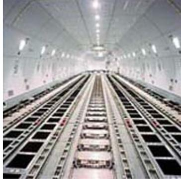
**Figura 7-34** Compartimiento o cabina principal del Boeing 747-400ER Freighter
