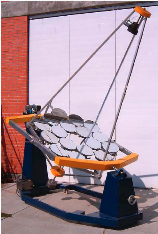
Fig. 2. DEFRACT (Spanish acronym of Device for the Study of Highly Concentrated Radiative Fluxes) [22].
