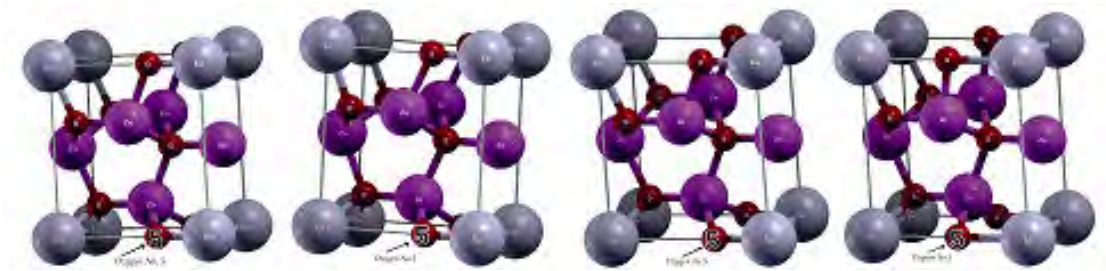
Fig.2. Oxygen 5 in its place, then it is out of place in x=0.45 a , 0.5 a , 0.55a . Where a is the lattice parameter.
