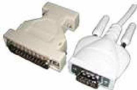
Figura 1-21 Conectores DB-25 y DB-9
