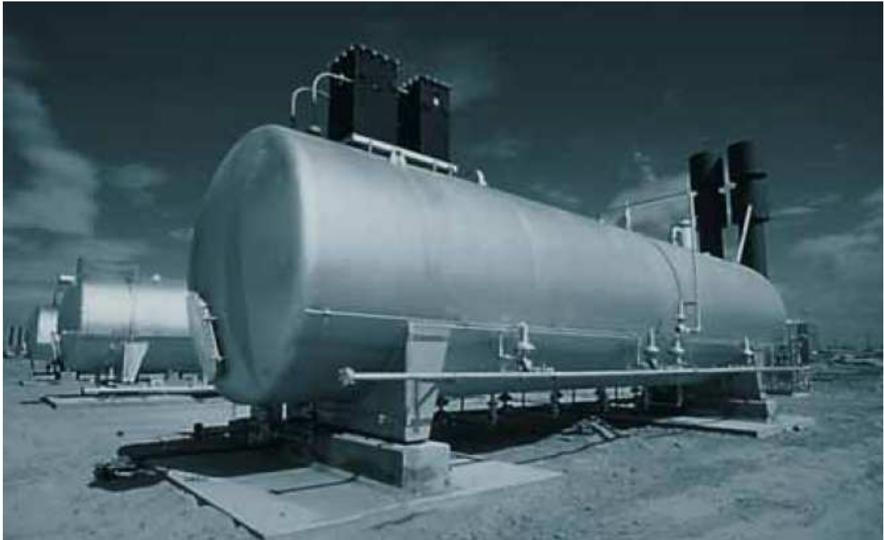
Figura 94: Tipico Tratador de Dual Polaridad Electrostatico Ref. Dual Polarity® Electrostatic Treater improves crude oil dehydration
