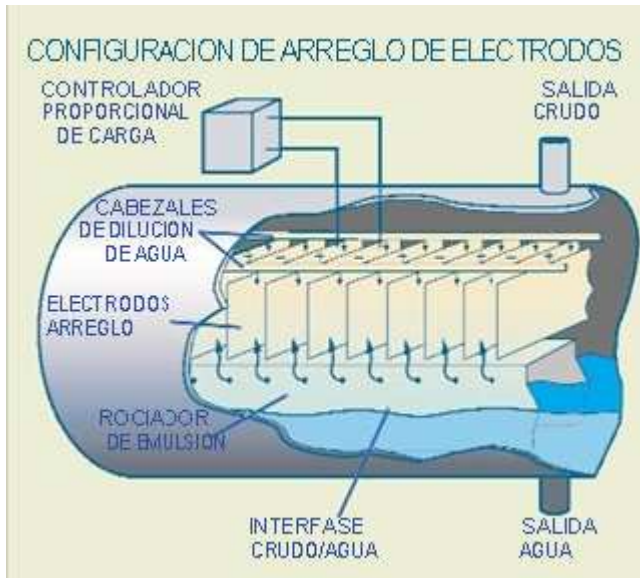
Figura No. 100 esquema de un desalador electrostático Ref. Electro-Dynamic@Desalter Field or Refinery: A Higher level of Desalting Performance
