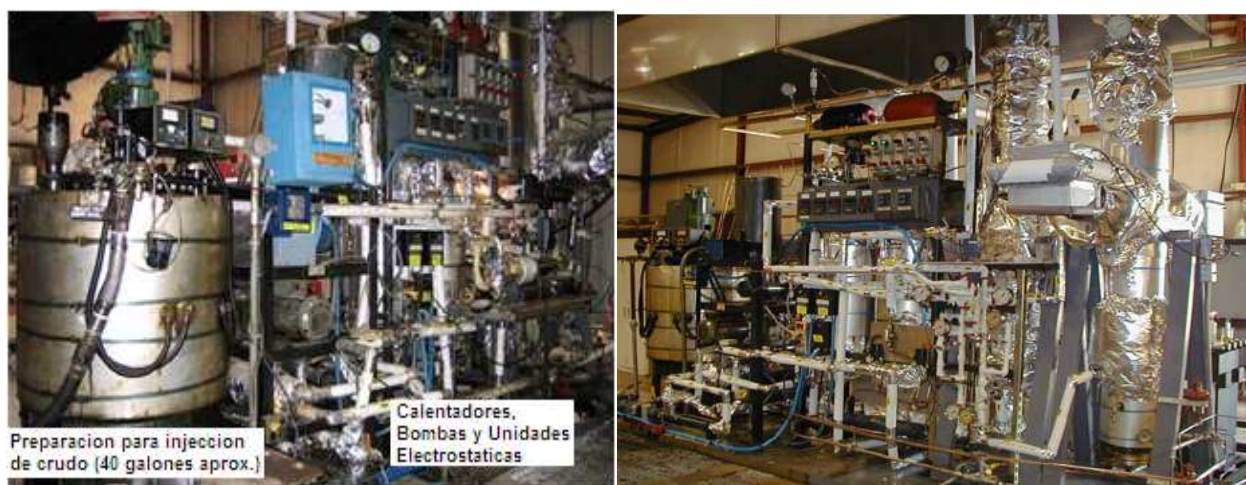
Figura 71: Deshidratador electrostático escala piloto (Natco). Ref. William H. Thomason/SPE, David J. Blumer/SPE, Probjot Singh/SPE, and David P. Cope, ConocoPhillips, and Moshen Zaouk, NATCO Advanced Electrostatic Technologies for Dehydration of Heavy Oils (2005))
