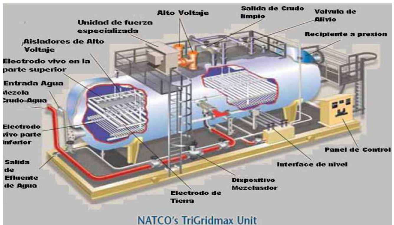
Figura No. 83 Detalle de deshidratador de AC Ref. TriGrid and TriGridmax Electrostatic Dehydrators/Desalters (Natco)
