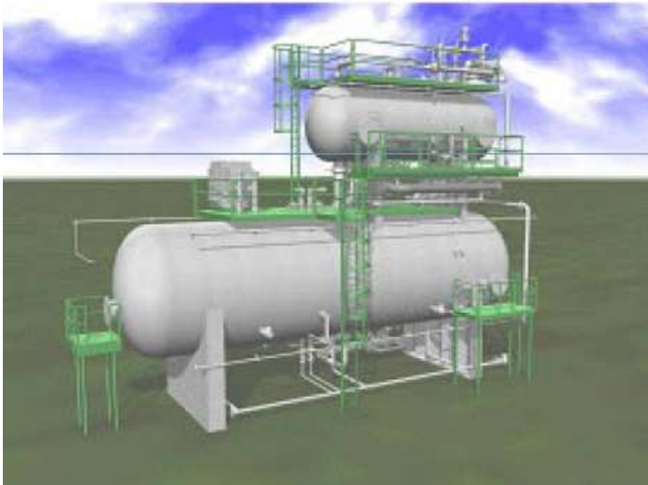
Figura 99: Esquema de un Desalador Electro dinamico Ref. Electro-Dynamic®Desalter Field or Refinery: A Higher level of Desalting Performance
