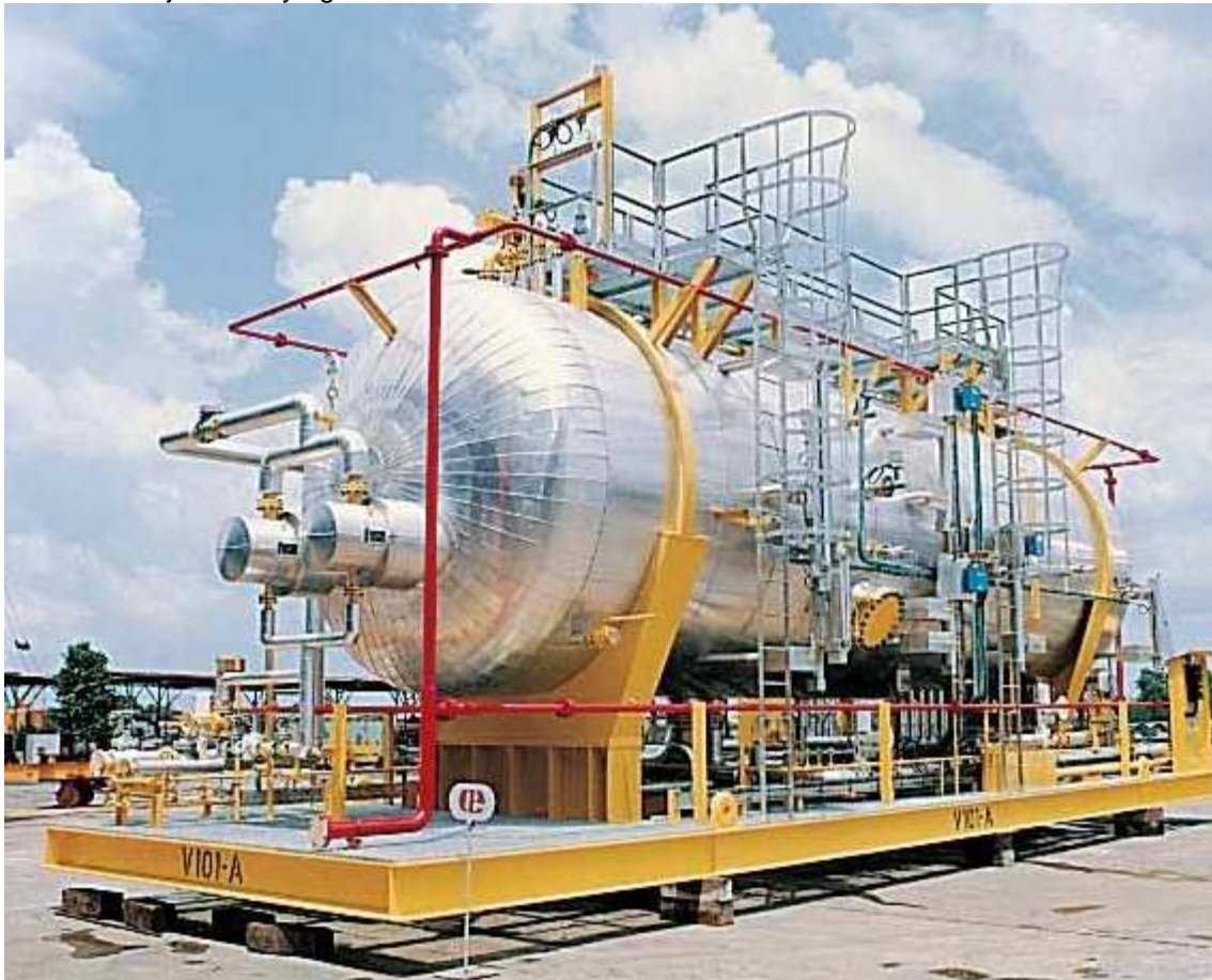
Fig No.82 15,000 bpd TriGridmax Desalador para Crudo Ashland en Nigeria Ref. TriGrid and TriGridmax Electrostatic Dehydrators and Desalters (Natco)
