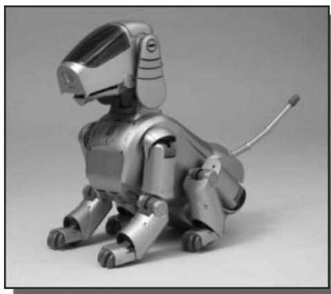
Fig. 1.15 Robot AIBO
