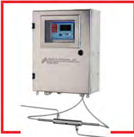
The **H2S-220** is a diode array UV fiber optics process spectrometer. It is designed to address on-line applications that require reliable, accurate, rugged and maintenance-free monitoring of H<sub>2</sub>S concentration. Either a fiber optics insitu probe or flow cell can be used.
