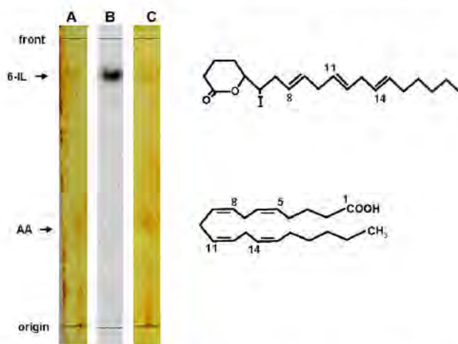
Fig. 1. Identification of 6-iodolactone (6-IL) and arachidonic acid (AA) by thin layer chromatography. Left panel: (A) 6- 125 I-IL and AA were visualized using iodine vapors; (B) 6- 125 I-IL was visualized using the Storm 860 phosphorimager scanner; (C) 6-IL and AA standards were visualized using iodine vapors. The samples contained 6 \mu g of lipids. Right panel: chemical structures of 6-IL and AA.
