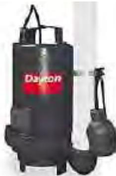
Effluent Pump, Submersible, Heavy Duty, 1/2 HP, Tether, Housing Cast Iron, Impeller Material Polypropylene, 230 Voltage, 5.1 Amps, Height 16 3/4 In., Dia. 12 1/4 In., Cord Length 20 Ft., Discharge NPT 2 In., Max. Dia. Solids 3/4 In., Max. Head 79 Ft., GPM of Water @ 50 Ft. of Head 36, Max. Temp. 104 F, Phase 1, Intermittent Duty
