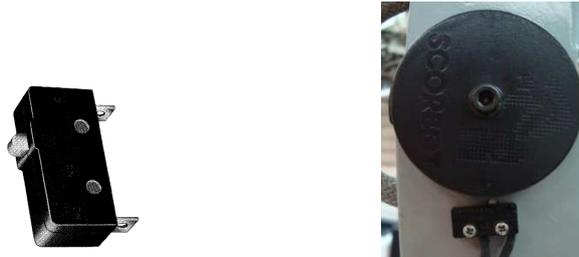
Figura 3.6. Micro-interruptor de Scorbot-ER V Plus
