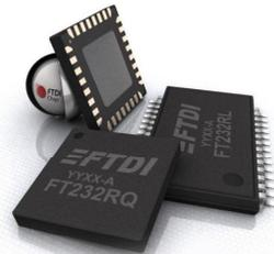
The FT232R is a USB to serial UART interface with the following advanced features:
