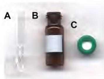
**Figure 10:** Insert, Vial, and Cap. Photo of conical insert A (Agilent PN 5181-1270), amber wide-opening vial B (Agilent PN 5182-0716), and screw cap C (Agilent PN 5182-0721), for amino acid analysis using the Agilent 1100 autosampler.
